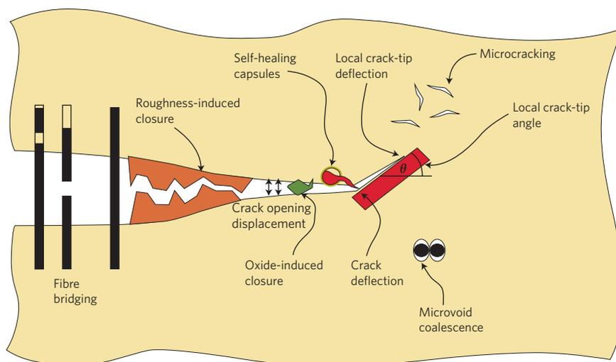
**Figure 2** | A wide range of toughening mechanisms can be observed and quantified by X-ray computed tomography, many of which are critical to the toughening of high-temperature ceramics. Image reproduced with permission from ref. 9, © 2012 AR.
