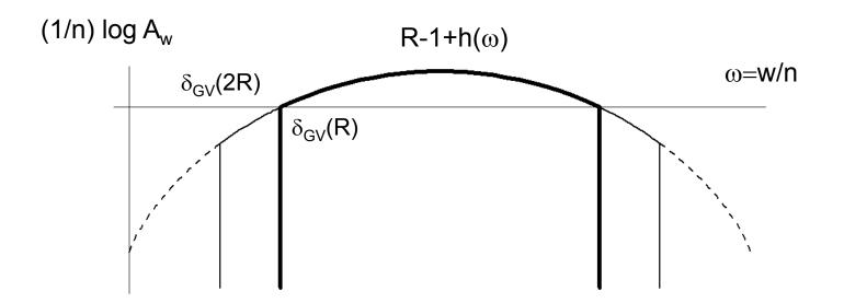
Bold curve: distance distribution of typical linear codes Solid curve: distance distribution of typical unrestricted code Dashed curve: average distance distribution of codes, linear or not
