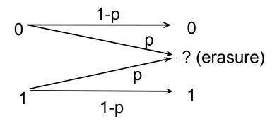
**Theorem 23.8:** The *capacity* of the erasure channel equals 1-p, attained by linear codes (For any R=1-p- $\epsilon$  there exists a sequence of linear codes of length  $n \rightarrow \infty$  for which the error prob. of decoding  $P_e \rightarrow 0$ ).
