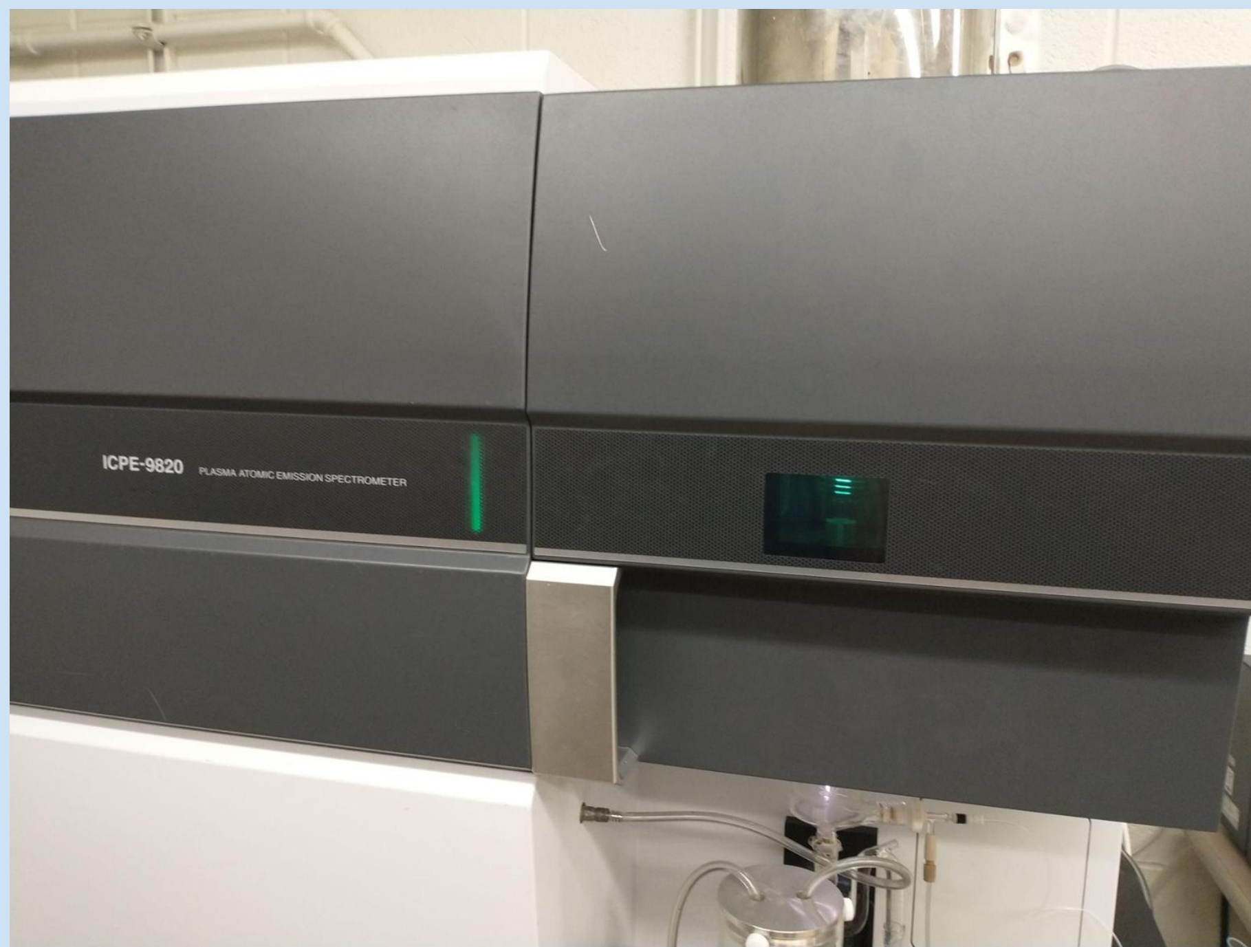
Photograph of the ICP-OES, an instrument in the lab used to determine trace element concentrations of water samples. Photographed by Alan Elliott.
