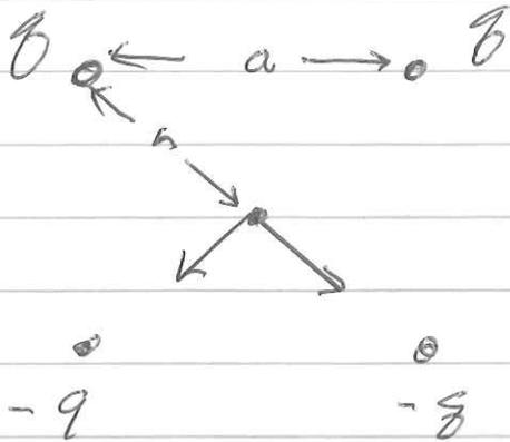
At the center the horizontal  $\vec{E}$  from the two positive  $q$ 's, and the two negative  $q$ 's cancels.  $\vec{E}$  is downward since  $\vec{E}$  from the positive and negative charges is down.
