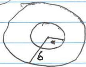
a) Material with resistivity  $\gamma$  between two radii. Use
