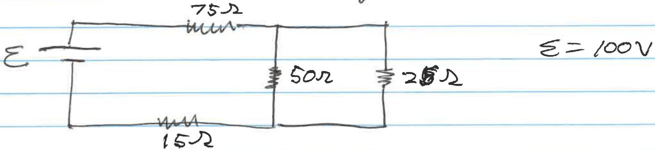
The right two resistors are in parallel
