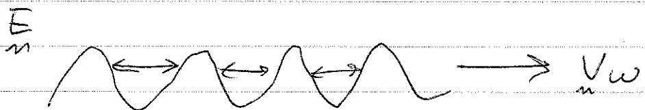
Particles can be trapped in the wave troughs, executing complicated orbits.
