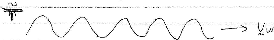
In sound waves  $\omega = kc_s$  so  $V_w \sim c_s \sim T^{\frac{1}{2}}$
