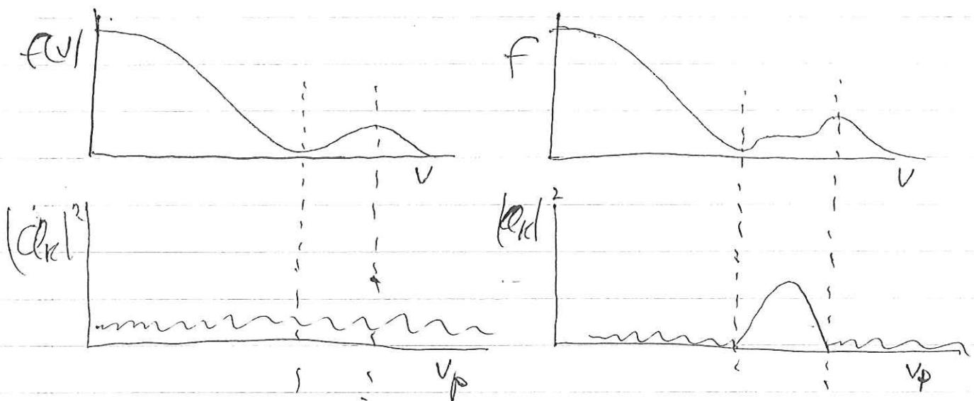
Resonant particles are dragged to smaller velocities, giving up energy to the waves
