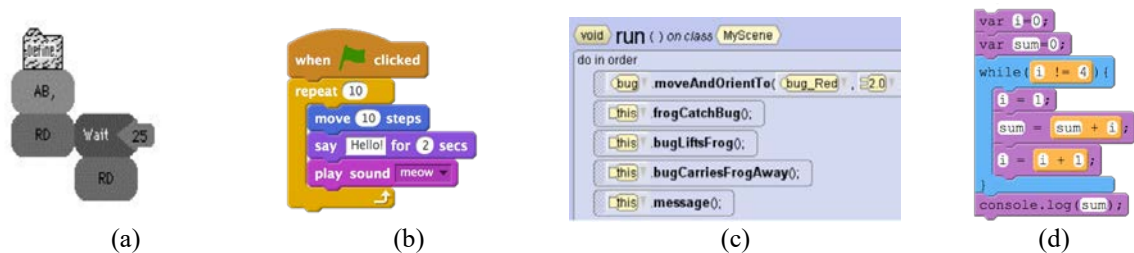
Figure 2. Block-based programming languages: (a) LogoBlocks, (b) Scratch, (c) Alice, and (d) Code.org's App Lab.
